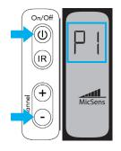
The correct microphone sensitivity ensures ideal sound quality for the receiver.
